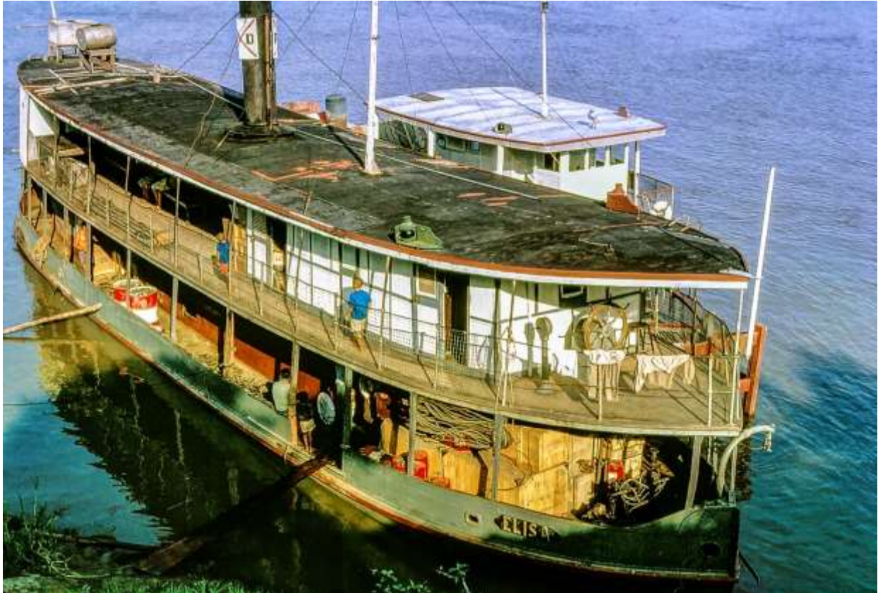
Amazon Riverboat "Elisa" when moored in Pucallpa. "Elisa" had no power of its own, it was propelled by a tug lashed to its side.
