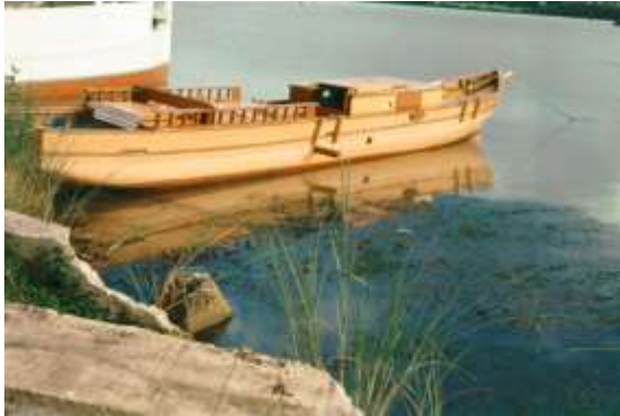
A cabin was built over the forward cargo hatch that gave 4-feet of head room. The supplies were stored in the aft cabin, where there was 3-feet of head room.
