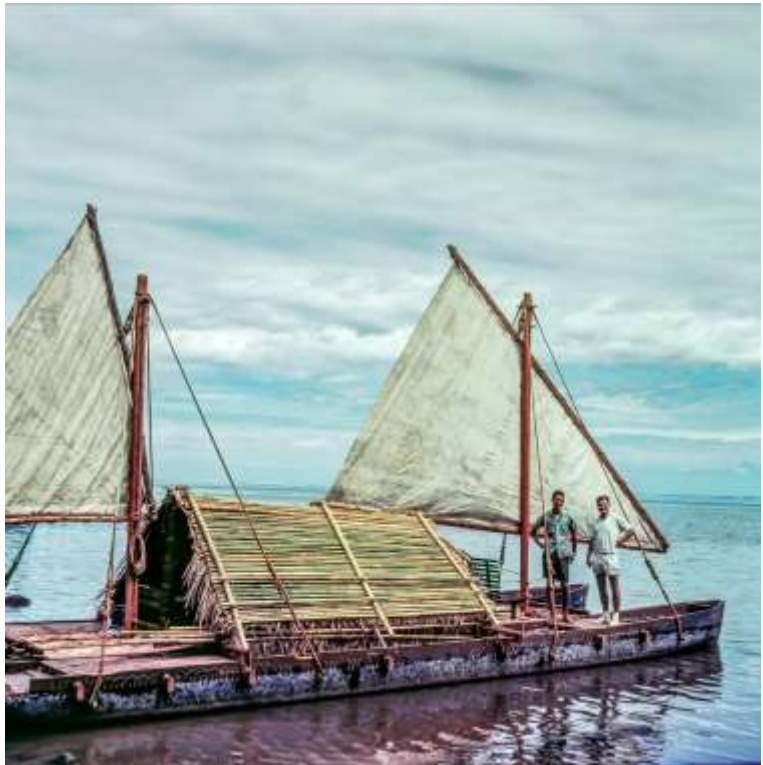
The completed Liki Tiki. On a trial sail, the large cabin area over powered the sails. I had to cut some of it away.
