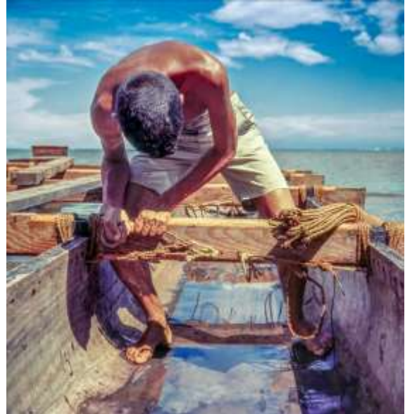
Lashing the cross beams to the canoes using coconut fiber rope.
